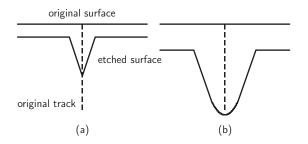
FIG. 12. Schematic of the etching process for two durations: (a) the etching time is not sufficient to reach the bottom of the original track; (b) rounding of the bottom of the pit after the track end has been reached.
