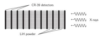
FIG. 11. Schematic of a sample unit composed of alternating layers of lithium-deuteride powder and plastic detectors (CR-39). The whole assembly includes several units like this, placed parallel to each other inside a hermetic PVC container. The distance between the detector plates is 1 cm. The total number of detectors in the whole assembly is 85. Each detector plate is a square of area  $1 \times 1$  cm with 1-mm thickness. The x rays are directed perpendicular to the plates.
